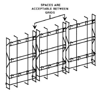
Determine the number of CI Conversion Grids (23 ¾"W x 35¼"H) required to fill the booth. For example, a 7'H x 10'W booth will require 5 Conversion Grids per row. Therefore, the two rows will require 10 Conversion Grids.
