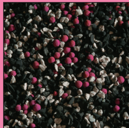
Triple Blend Media with Activated Carbon, Impregnated Alumina and Zeolite.
